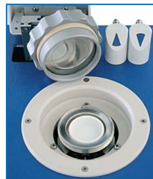
stainless steel chamber with PTFE-sample dish
