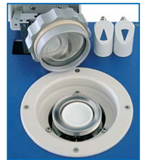
stainless steel chamber with PTFE-sample dish
